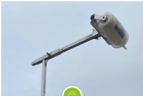
**BLADE TIP HOLDER** Working at the tip is the most vibrating experience in the total operation. To minimize this vibration and provide stable support, we offer blade tip holders.
