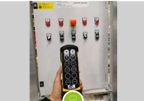
**REMOTE CONTROL** The K-BP-2L can be operated using a remote control. We also provide a control panel on the control box in case of remote control loss or damage.
