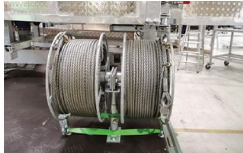
**ROPE CAROUSEL** We provide this carousel where 4 x 10 mm ropes are wound to make rope installation easier and faster. It is also helpful when ropes get mingled.
